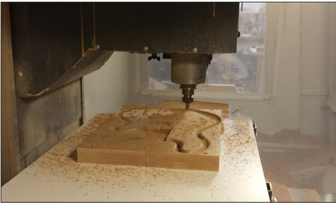
Vacuum workholding systems allow several complex operations to be performed in a single setup. Here a guitar body is routed from dense hardwood stock without clamps.
