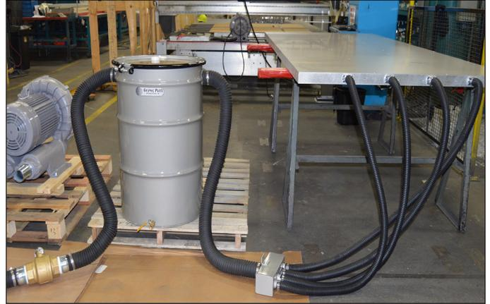
A simple vacuum table system for an industrial application, including vacuum table with perforated surface, multiple ports, manifold, coolant collection barrel, shut-off valve, and vacuum pump.
