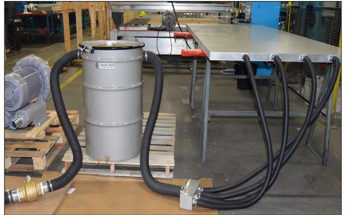
A simple vacuum table system for an industrial application, including vacuum table with perforated surface, multiple ports, manifold, coolant collection barrel, shut-off valve, and vacuum pump.
